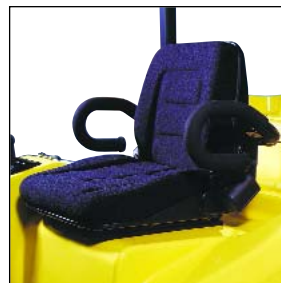
Adjustable semi-suspension seat with retractable seat belts.
