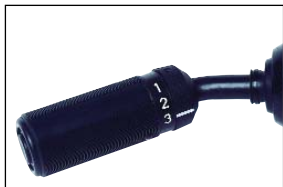
Directional/gear-shift lever located on steering column.
