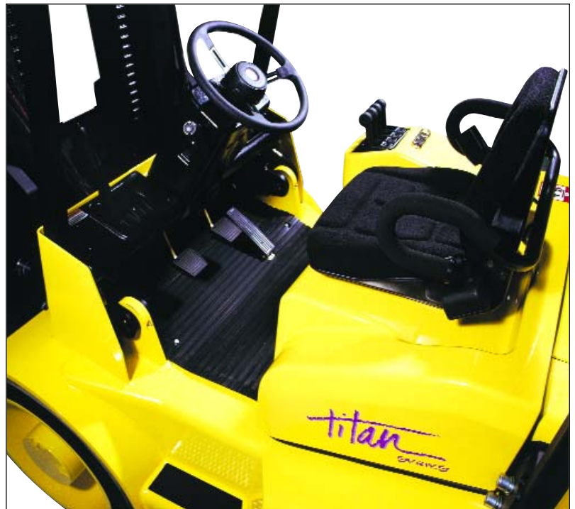
The operator platform meets ANSI B56.1 FOPS operator protection.
