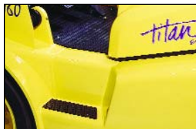
Low, 18-inch, non-skid steps for safe and easy entry and exit.
