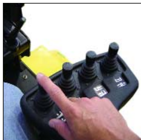
Optional finger-tip levers are designed to move within the full range of seating positions.
