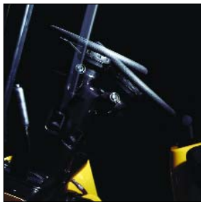
Tilt-steering column. Easy entry and exit for any size operator.
